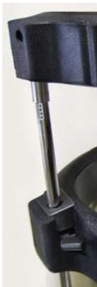
Fig. 2: Spring scale on a rod of the Vertetrac
