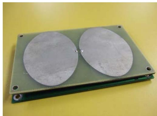
Fig. 5: The UWB radar sensor
